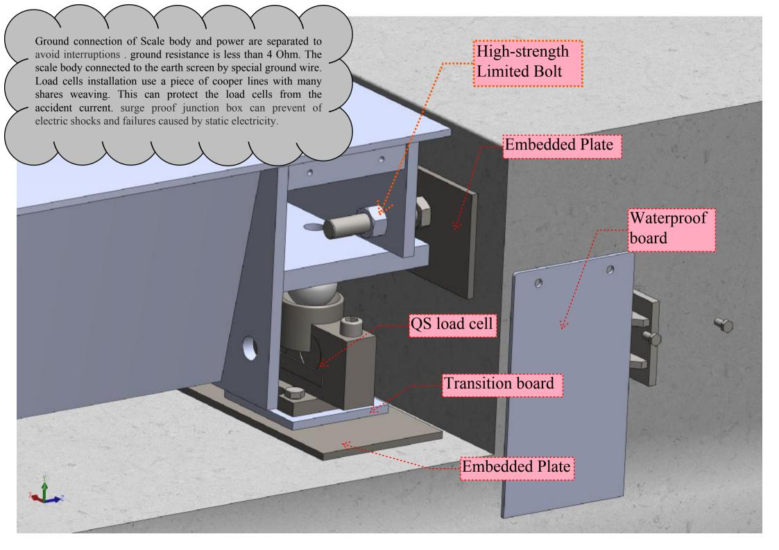
Limited Board (Welded on the embedded Plate) Attention:keep 3mm gap with scale body
